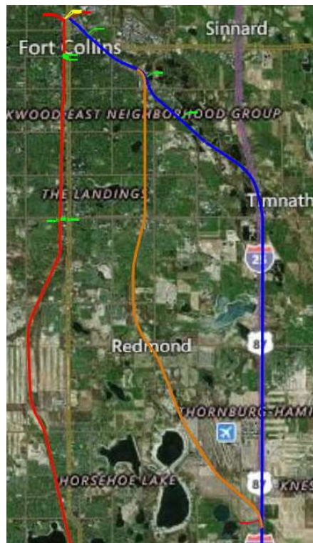
Figure 7. The orange alignment follows an existing UP freight corridor.
